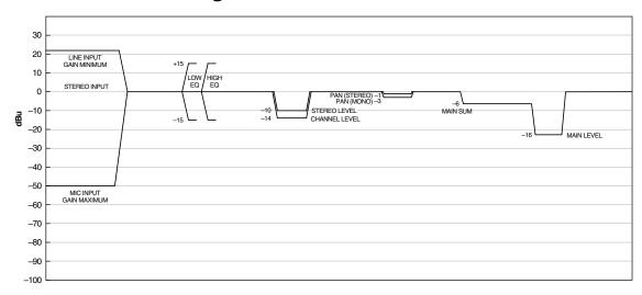
This diagram shows the gain levels in dBu, and the range of adjustment of the signal level as it wanders through the various circuitry inside the mixer. The left side is the input, where the signals enter the mixer, and the right side is the main output.
